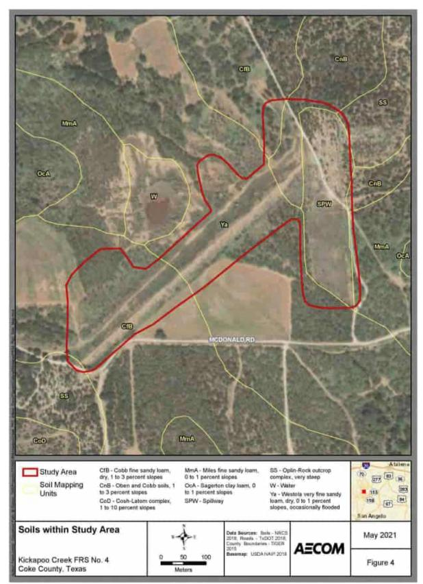
Figure 4. Soils within the FRS No. 4 Study Area
